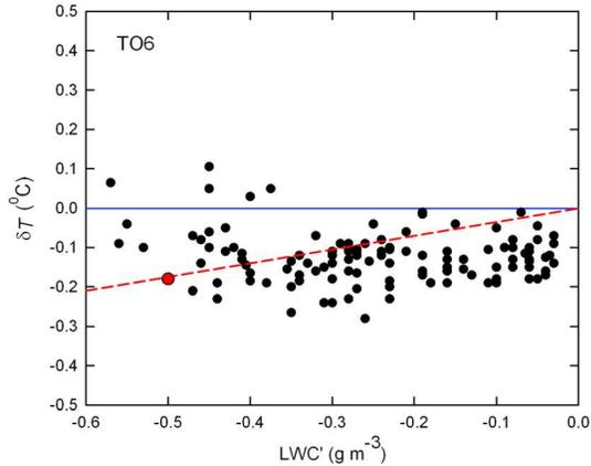
**Figure 15.** The temperature change  $\delta T_m$  in cloud holes (black circles) corresponding to the maximum value of depleted liquid water content  $LWC'$  found in each hole for flight TO6. The red circle and dashed line indicate predictions from mixture fraction analysis for evaporative cooling (see text).
