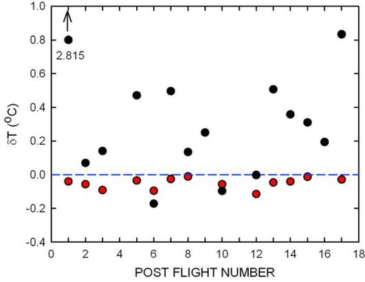
**Figure 13.** The temperature change ( $\delta T_p$ , black circles) predicted by mixture fraction analysis for POST flights, and the mean measured temperature change ( $\delta T_m$ , red circles) in cloud holes for POST flights (see text and Table 4).
