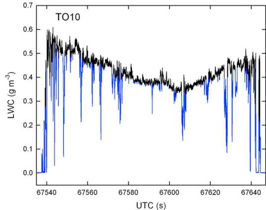
**Figure 4.** One porpoise down and up through  $\sim 100 \text{ m}$  of the Sc on flight TO10 showing 50 Hz LWC (black line) as a function of flight time. Cloud holes with narrow regions of reduced LWC (blue lines) are chosen by conditional sampling and are assumed to form by the entrainment process.
