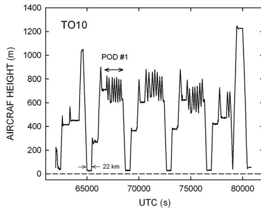
**Figure 3.** Vertical flight path of the Twin Otter aircraft during flight TO10. During the sawtooth patterns, given the name “pods,” the aircraft flew slant paths profiles (porpoises) 100 m above and below cloud top. Horizontal legs  $\sim 22$  km long were flown near the sea surface, just below cloud base, and within the cloud.
