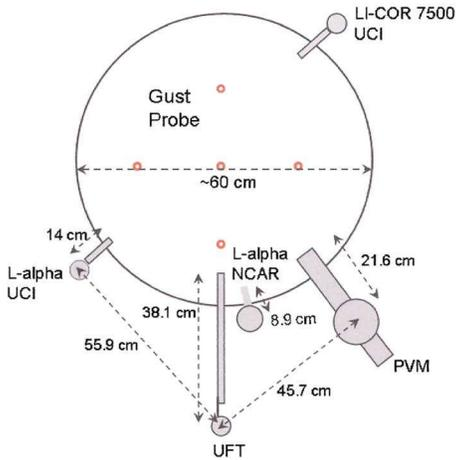
**Figure 1.** Head-on view of the CIRPAS Twin Otter (TO) research aircraft showing the locations of the UFT-M and PVM probes, and the Lyman-alpha probes which surround the UCI five-hole gust probe on the aircraft’s nose.
