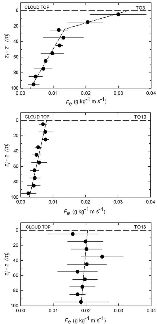
**Figure 8.** Average values of the entrainment mass flux  $F_e$  as a function of height below cloud top ( $z_i - z$ ) for flights TO3, TO10, and TO13. Horizontal lines are  $\pm 1$  standard deviation of the  $F_e$  measurements. Dashed lines are linear regression fits to the data.
