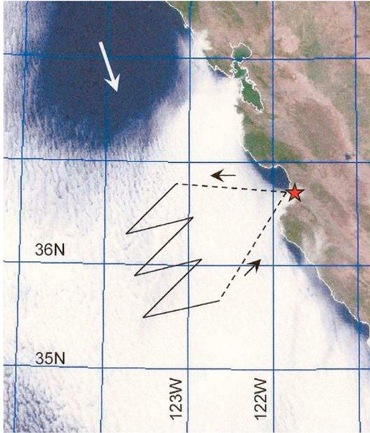
**Figure 2.** Early evening NexSat image (courtesy of the Naval Research Laboratory, Monterey) off the CA coast and the Pacific Ocean showing the approximate track of the Twin Otter aircraft on flight TO3 (19 July, UTC). The red star indicates the location of Marina airport near Monterey Bay, and the white arrow is the prevailing wind direction at cloud level. The Sc is dissipating upwind from the track.
